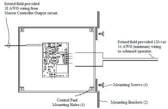
Wiring the Remote Operator: This unit is not provided with a power supply. Only connect 24-vac from an approved source at the input terminals on the pc board. Connect 24-vac cable from Master Controller as shown. For Units operating 120-vac devices, 120-vac line should be routed from power source through terminals as shown. Neutral can be routed separate from the wiring at this unit. Extend 24-vac to device as shown where the control is 24-vac.
